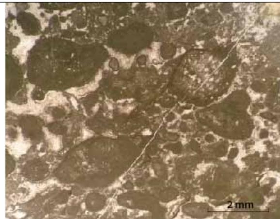
Figure 4. Oncolitic packstone, sample 3145. / Figura 4. Packstone oncolitic, proba 3145 (original).
