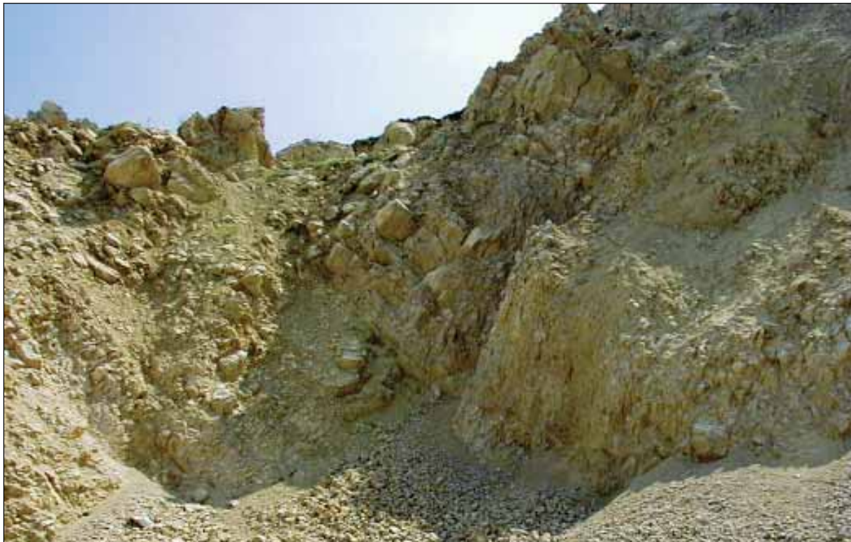
Figure 1. Strongly fractured limestone including some sandstone and clay contamination. Figura 1. Calcar intens fracturat contaminat cu gresii și argile (original).
