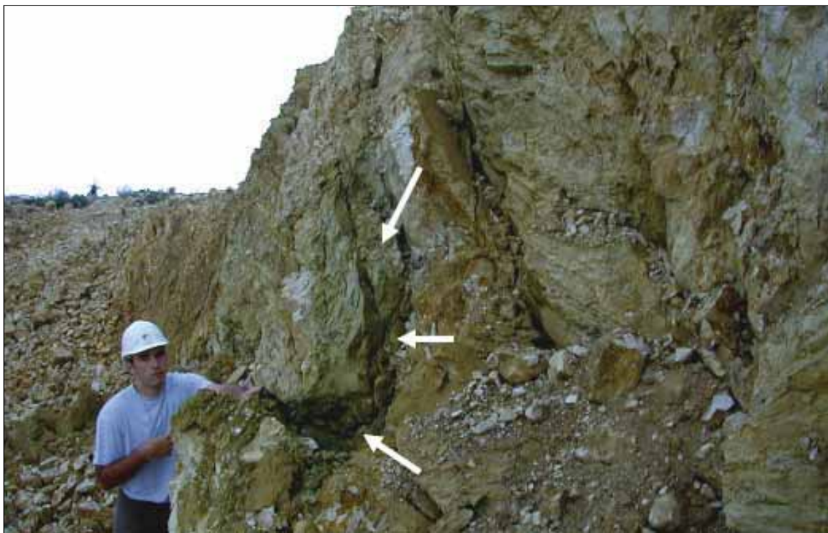
Figure 4. Smeared the clastic sediments into the faults with green clay (endokarst). Figura 4. Contaminarea fracturilor din calcar cu umpluturi carstice de argile verzi (endocarst) (original).
