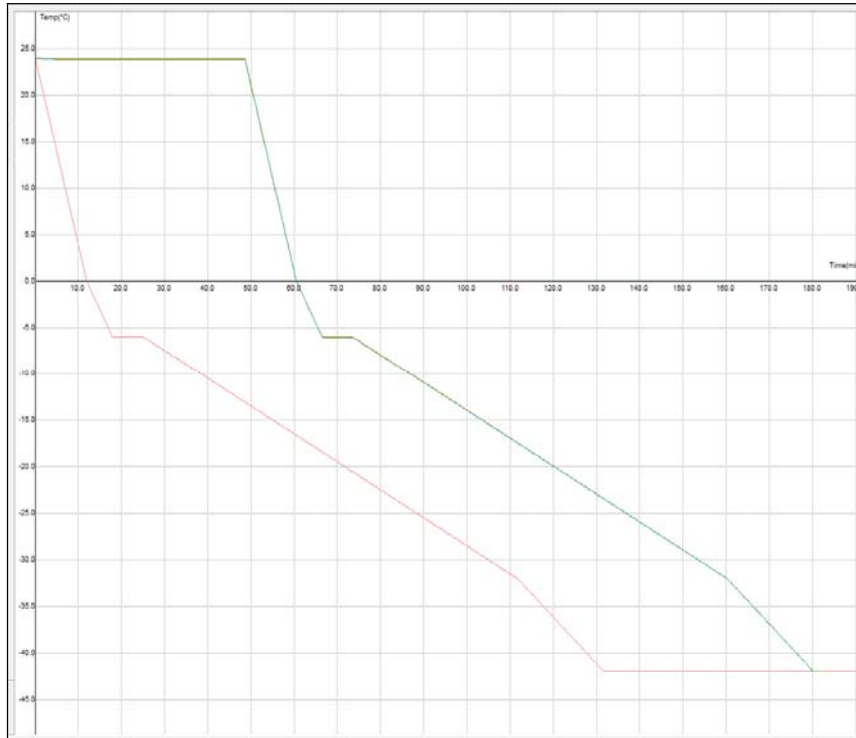
Figure 1. Slow freezing temperature graphic (CryoGenesis 5). Y-temperature (°C), X-time (minutes); red line-protocol parameters, green line-achieved parameters.
