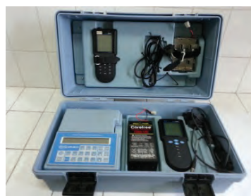
Figure 6. Portable kit for determining the water analysis in situ.
