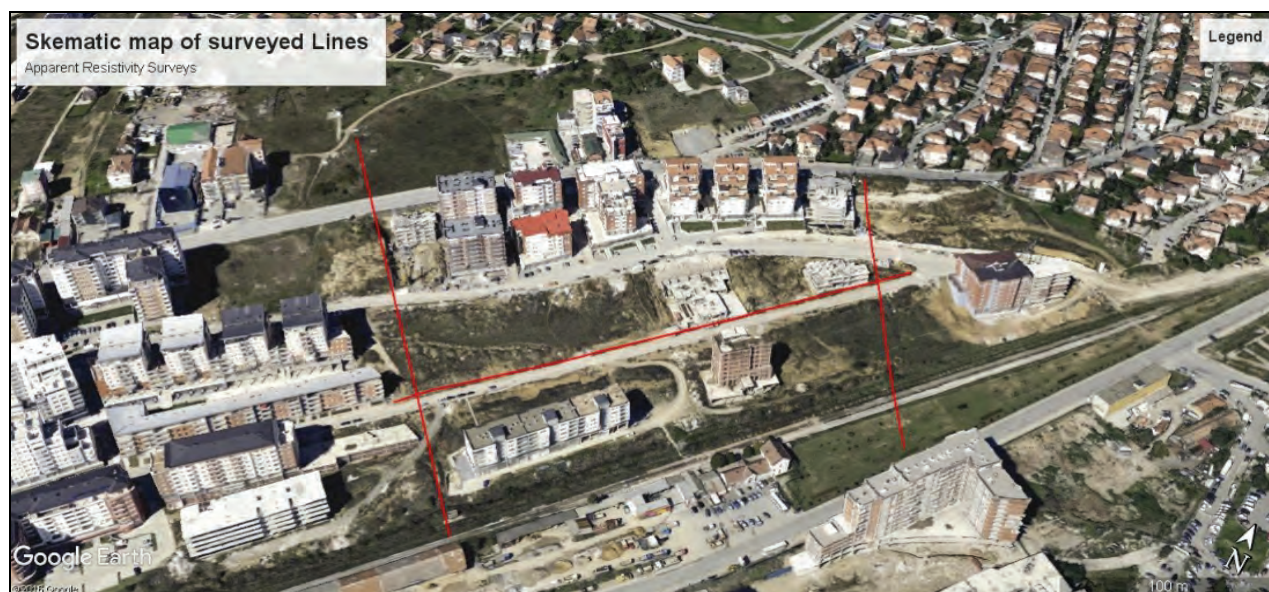
Figure 1. Schematic map of the surveyed area and proposed survey lines (Google Earth, modified by Karriqi).
